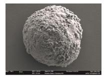
SEM image of a microtissue produced at the ICBC in Wädenswil. These tissues have been made by applying the hanging-drop method and consist of human colon cancer cells.
