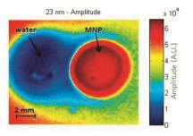
Thermographic amplitude image. The image shows two drops consisting of distilled water, where one is treated with magnetic nanoparticles (Fe3O4). The particles lead to distinct heat emissions.
