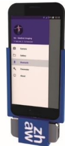
Developed Android application intended to overlay a thermogram from IR-camera FLIR ONE with an optical image from smartphone camera. The smartphone case integrates a laser sensor in order to measure the distance to the object.
