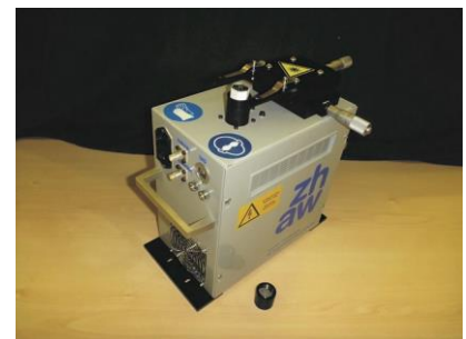
A first prototype of the developed excitation device for gold nanorods
