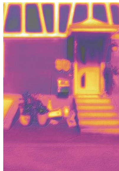
Overlay of the smartphone image and the infrared image of the Flir One
