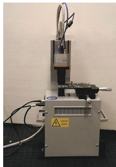
Optimized multispectral LED-based excitation device
