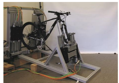
Fahrradsimulator am Institut IMES - Biomechanical Engineering
