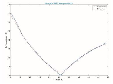
Comparison of the surface temperature of the human skin as simulation with experimental data. The simulation was performed with the numerical thermal model. The Experiment was realised during a clinical study at Geneva University Hospital.
