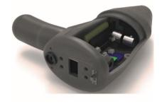
Developed prototype. With this handheld device it is possible to perform a thermographic examination.
