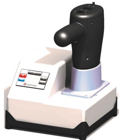
Coolingstation prototype including a provisional cameramount and camera as a placeholder.
