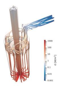
Simulated particle paths through an irradiated reactor. When combined with the power density G, the UV dose of the particles can be calculated.
