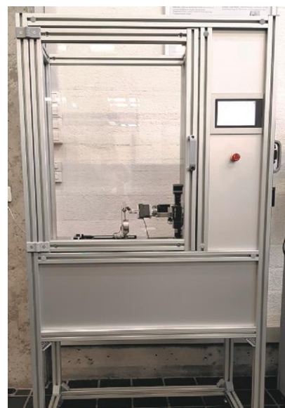
Picture 1: Manometer Calibration Station (Frontal View)
