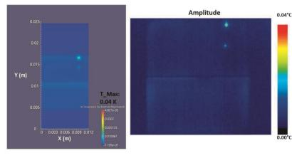
Small-signal DLIT simulation (left) and measurement (right) showing the temperature amplitude of a perovskite dua cell with two shunts in the upper cell and a interconnection in the center. The simulati allows to better understand the nature of t defects and to quantify them.
